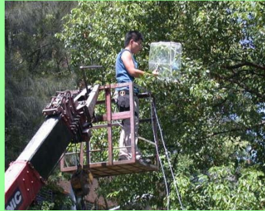
Figure 2. Technician with the chamber hoisted to the branches selected for Vd measurements.
