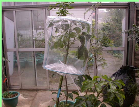
The branch enclosure chamber for fast screening of high NO 2 uptake trees
