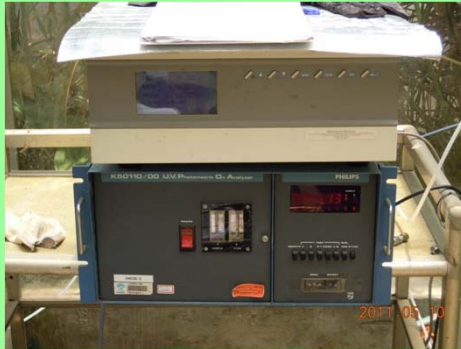
Eco-tech NO 2 monitor and Phillips Ozone monitor
