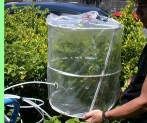
The branch enclosure chamber for fast screening of high NO 2 uptake trees
