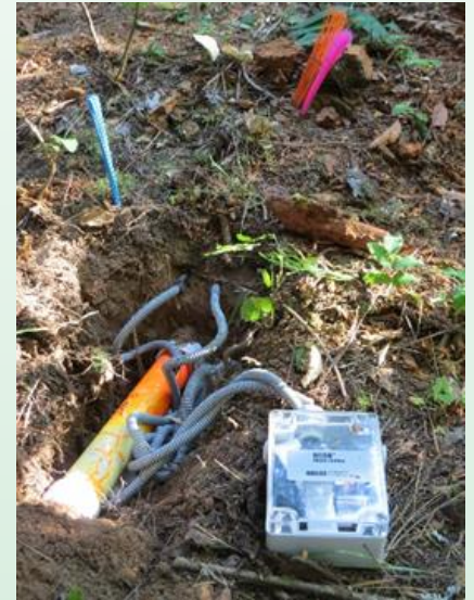
Installing soil temperature and moisture probes
